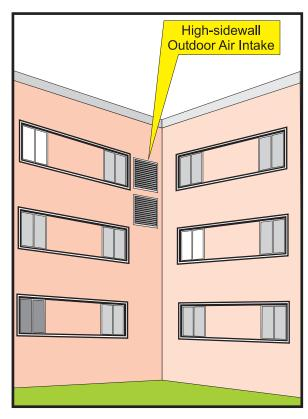
architecturally compatible design. The goal is to minimize public accessibility. In general, this means the higher the exten*sions. the better*—as long as other design constraints (excessive pressure loss, dynamic and static loads on structure) are appropriately considered. An extension height of 12 feet (3.7 m) will place the intake out of reach of individuals without some assistance. Also. the entrance to the intake should be covered with a sloped metal mesh to reduce
